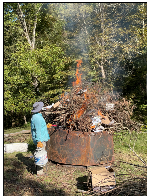
Dr. Amir Hass ignites the materials in the kiln which will burn to create biochar.
