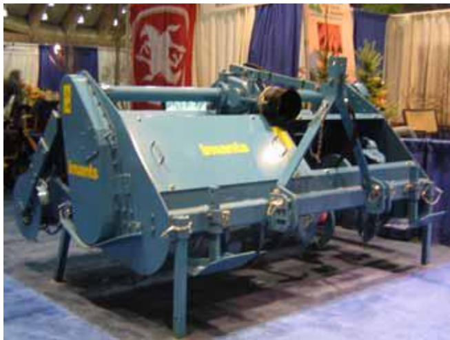
This large rototiller appears to be able to till as much as 18" deep.
