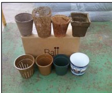
Front row (left to right): Slotted Rice Hull, Solid Rice Hull, Plastic (conventional), SoilWrap (PHA plastic)
